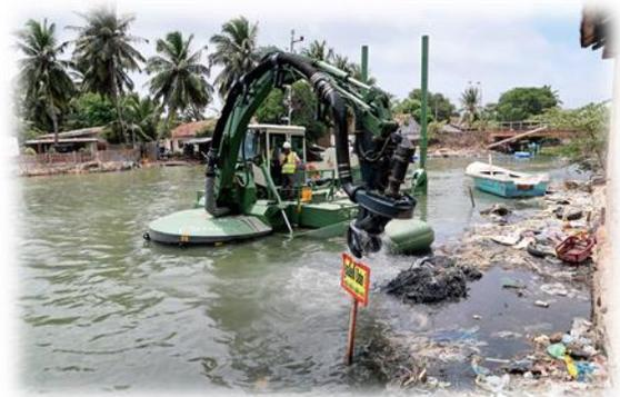
The **new hard soil cutter crown** together with the **bigger, more powerful hydraulic motor** take Watermaster Classic V to a **new capacity level in hard soil dredging**, too.
