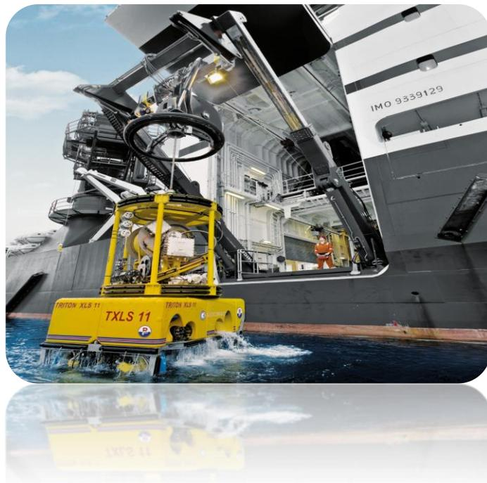
Each system measures ship movement and relays the data to a main controller. The controller then uses that information to control other components, which in turn power the winch so that the load hangs idle relative to the fixed world (i.e., the drilling rig or the seabed). So when the ship moves upwards, the winch pays out; when it comes down again, the winch hauls in. This makes it possible to position loads accurately and safely, even in rough weather.
