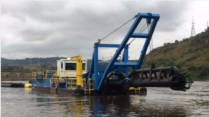
Rohr-Idreco RISD 600 (24") 100' digging depth dredge for removal of sedimentation behind the Inga dam in the Democratic Republic of Congo
