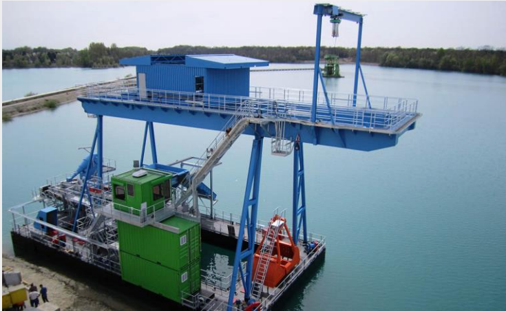
In the foreground is a new Floating Gantry Clamshell dredge. In the background - a 32 year old Gantry Clamshell, which was refurbished and is now back in operation.
