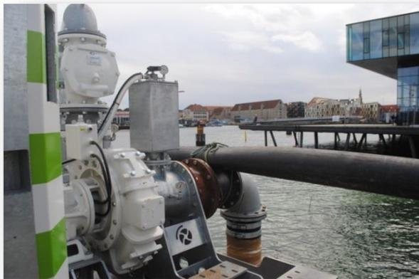
Rather than with earthmoving equipment, the actual digging is done with a submersible Damen pump that is suspended from an excavator or crane. By installing jetting nozzles on the submersible pump the soil is agitated, creating a slurry that can be pumped away, thereby digging out the soil. When the intended depth is reached, underwater concrete is poured to create a watertight base that will create a caisson in combination with the
