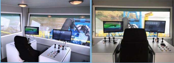
*Operator cabin with Dredge Control & Digital GPS Sonar Systems with map & digital screen read outs*
