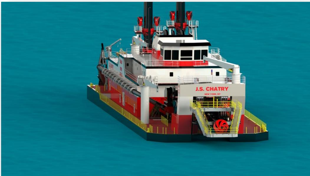
cutterhead. When the dredge is not offshore, it is equipped with a walking spud carriage for efficient work in inlets and in protected waters. 52 people can be comfortably housed onboard.
