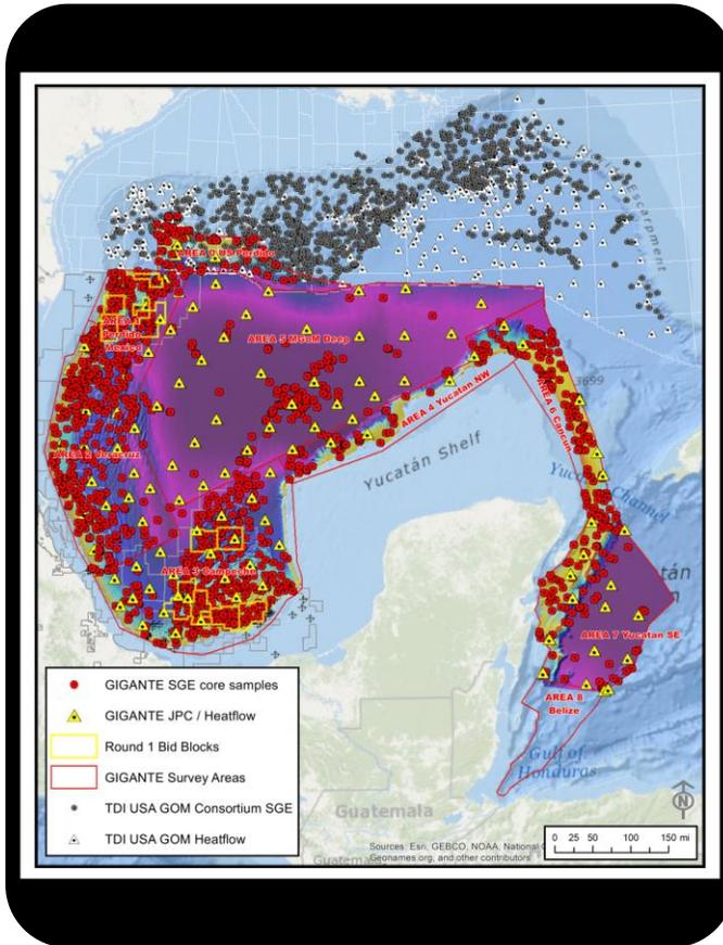
TDI-Brooks International, Inc (under contract to TGS), recently completed an exploration geochemistry program in the Southern Gulf of Mexico consisting of 1,180 USBL positioned piston cores for geochemistry, with an additional 120 heat flow measurements for basin modelling and 120 20m “jumbo” piston cores for stratigraphic analysis and age dating.
