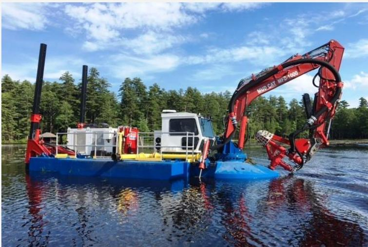
*Griffin and Howe's Mud Cat MFD utilizing the MC-Cutter Pump attachment to deepen Echo Lake.*
