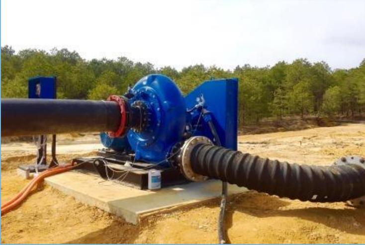
*With the addition of the RI booster pump, the dredging system now exceeds plant capacity of 400tph*
