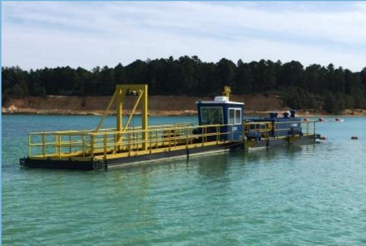
*The Rohr-Idreco RISD300-M (12") electric dredge for sand & gravel application*
