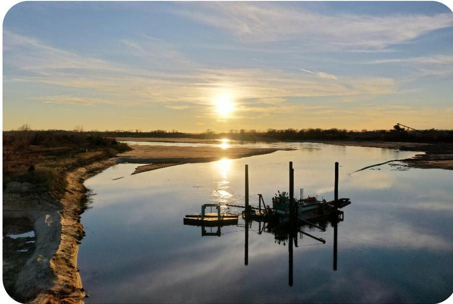
The SHARKUDA® Dredge Class is designed to excel in areas otherwise difficult to access; it incorporates two newly patented technologies: the new walking carriages which allow the dredge to continually move forward without anchors for continuous, uninterrupted production; and the new swinging ladder which allows for wide deep swings to operate more efficiently than any other conventional dredge on the market.
