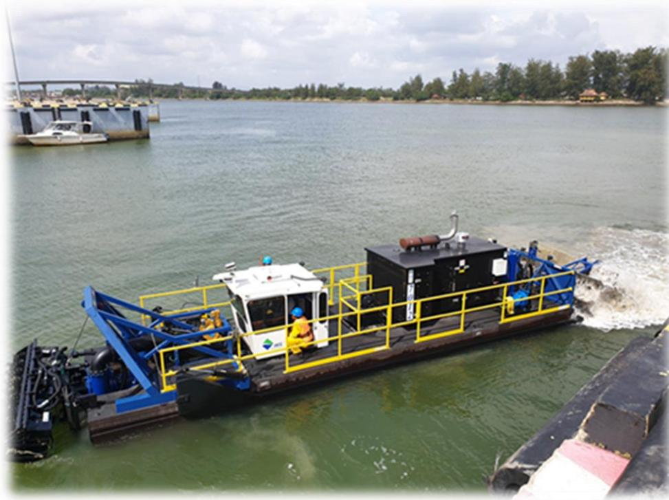
*The 7012 HP JetMaster® dredge maneuvers itself into the dredging area with its patented Starwheel Drive self-propulsion system*
