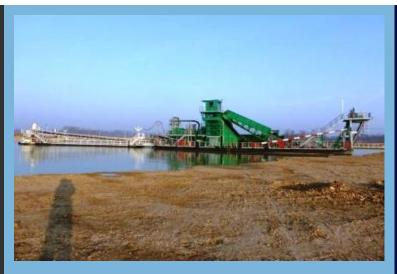
Rohr's floating bucket ladders have a standard digging depth of up to 60 ft. (18m), but can be designed to reach up to 75 ft. (23m) Production ranges from 300 to over 1,000 tph, depending on material and digging depth.
